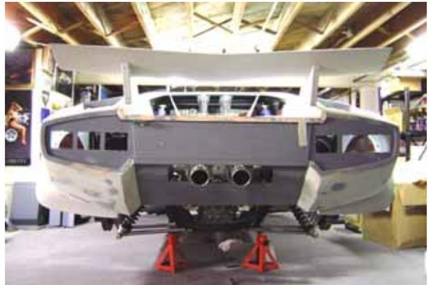
“Here are the pictures of the chassis. A full tube frame supporting the aluminum body. Hand built stainless steel 180 deg. headers with 12”long racing mufflers. All Corvette design suspension replaced with steel tube and rod ends for adjustments on caster, chamber and toe. Aluminum radiators with 2400cfm puller fans set to turn on at 180 degs or an override switch on the dash. 4 piston Wilwood calipers on 12” rotors. Full adjustable front and rear sway bars, and coil over shocks.”
