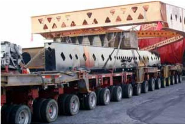
Here you can see how the immense weight was distributed across the trailer sections as well as the hinge points for the support bridge. Both ends are supported in this fashion, making the whole rig a lot more flexible than it might first appear. Those outriggers I mentioned are clearly visible along the outer edge of the trailer.
