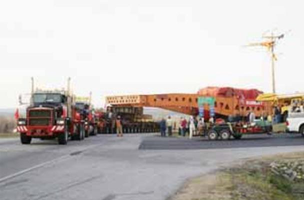
As things advance, dozens of power crews are on hand to clear overhead wires and there are hundreds of other support crews and dozens of support trucks waiting to fall in line behind the convoy. Notice that each large truck has a box firmly anchored over the rear wheels. Those are 18,500 pound weights which give the truck the
