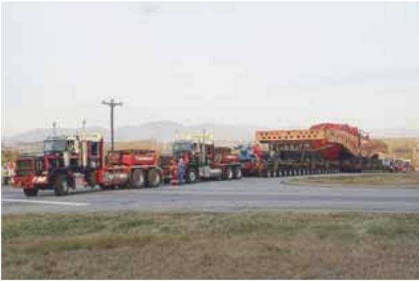
Here is the rig I'm talking about.... The trailer, as rigged, is 300 ft. long all by itself. There are 36 rows of axles, each with 8 tires. (288 total) These can be augmented with up to another additional 80 wheels on hinged outriggers, for a total of 368 potential flats. Add in 5 each 10 wheel heavy duty road tractors (2 pulling and 3 pushing) and that flat tire potential rises to 418. The outriggers are not deployed in these photos, so the total tire count, for the moment, is 338.
