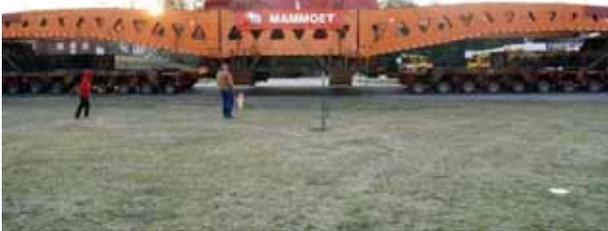
The main bridge beams suspend the huge generator about 18 inches above the roadbed. When the job is completed, the round pins near the bottom edge can be removed and the beams can be stacked for their return trip home. Even up close they almost look too small to be holding that much weight up in the air. Standing near this beam is a little spooky. All kinds of pops and groans can be heard, even when it isn't on the move.
