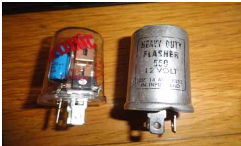
New electronic on left and older thermal type on right
