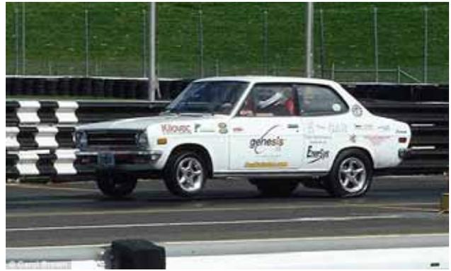
And she's off: Nicknamed White Zombie, the Datsun can go 90 miles without being recharged and its 500 horsepower means it can cover a quarter of a mile in just ten seconds
