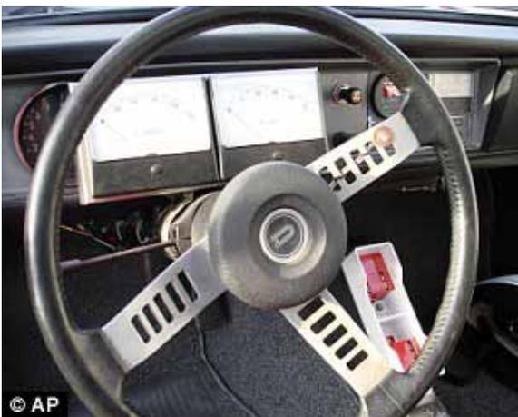
Hi-tech: The dashboard shows amps and volts generated by the electric car's batteries, while the boot houses the lithium-ion battery pack
