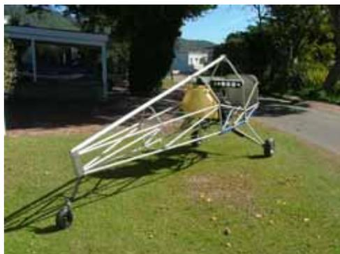
Technical specification, wingspan 9.0 mtrs, length 5.2 metres, empty weight 145 kgs, maximum gross weight with fuel and pilot 270 kgs. Power plant is a Rotax 503 of 42 hp running a three-blade ground adjustable prop through a 2.58 to one gearbox.
