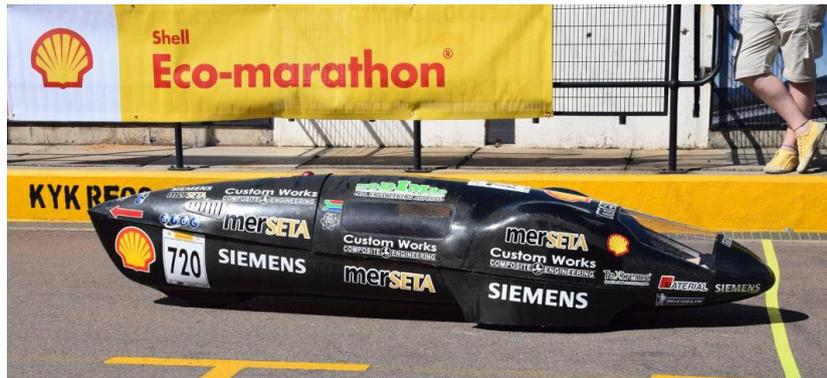
“Designed and built by students of the Nelson Mandela Metropolitan University, it’s an ultra-light, fuel efficient, carbon-composite vehicle powered by a 125 cc, fuel-injected, 4-stroke engine that boasts a measured fuel efficiency of 127,86 km/l of ordinary unleaded petrol – which would make it capable of travelling 6,393 km on standard 50 litre tank (or about the distance from Johannesburg to Cairo),” said Mr. Pretorius.
